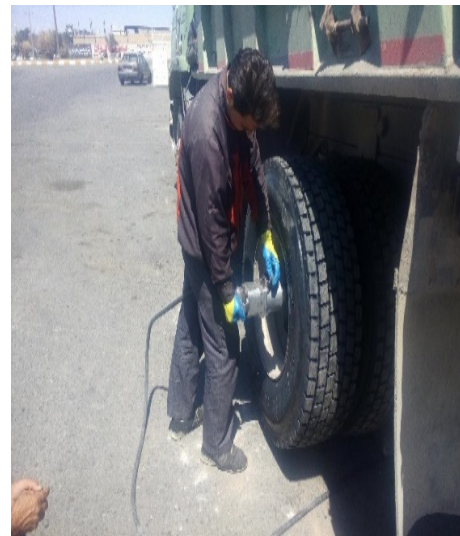
Figure 1. Pneumatic wrench on the left, a worker using it on the right
