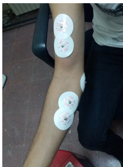
Figure 1: Location of electrodes on biceps and flexor muscles and reference electrode in the study
