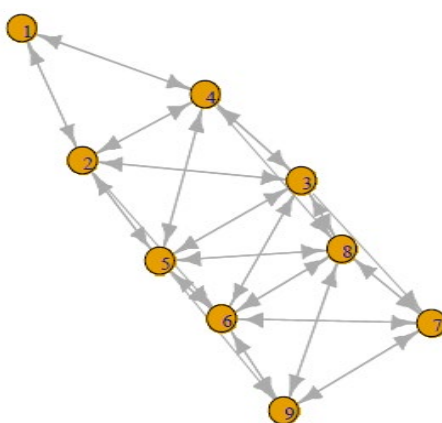
Fig. 1. Graph modeling corresponding to domino scenarios in the studied tanks, using R software.
