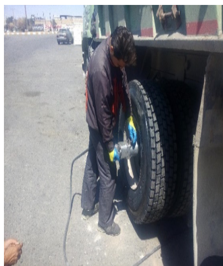
Figure 1. Pneumatic wrench on the left, a worker using it on the right
